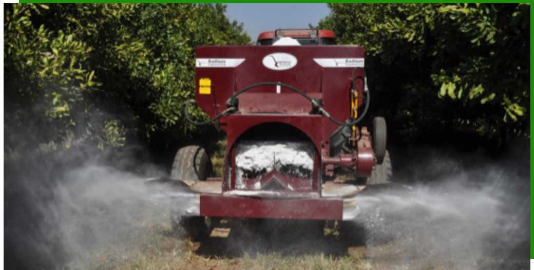
Side delivery attachment for under-tree fertiliser banding
