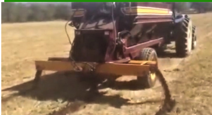
Band – spreader attachment for row crops and under plastic mulch
